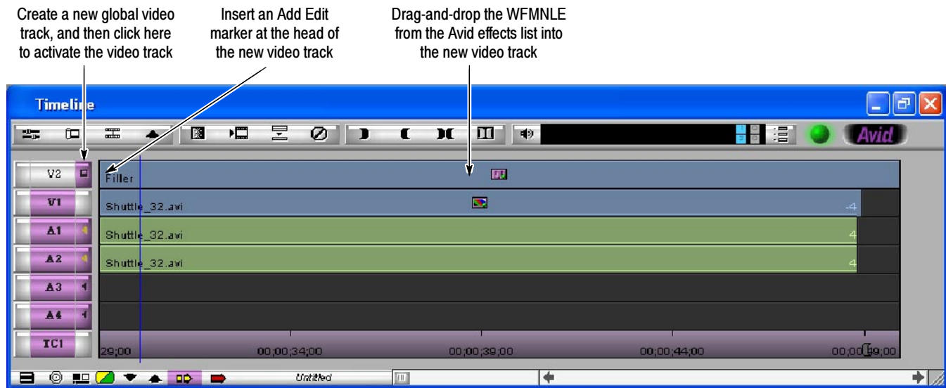
Figure 2: Starting the WFMNLE Software Waveform Monitor in an Avid Timeline window
